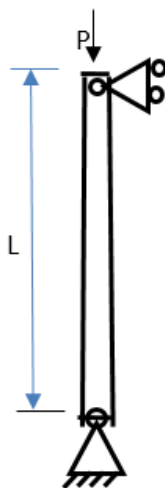
Figure 1 Parameters involved in the buckling of an element
