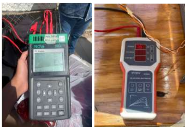
Figure 9 Equipment for measuring the electrical parameters of photovoltaic modules Own Source
