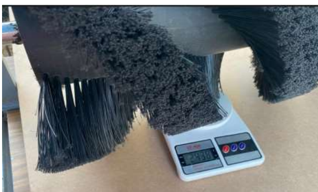
Figure 6 Experimental tests to obtain the pressure exerted by the roller on a Surface Own Source
