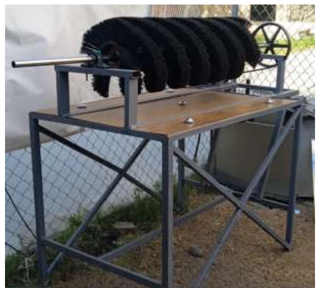
Figure 11 Final prototype of a dry cleaning system for photovoltaic modules Own Source
