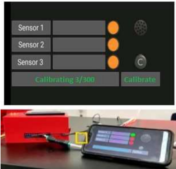
Figure 3 CO 2 monitoring system, implemented in a box and the App on a cell phone
