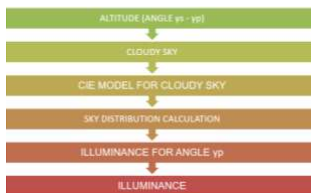
Figure 3 Schematic for calculating daylight availability ( \gamma_s solar altitude, \gamma_p altitude angle path in the sky), for cloudy sky. CIE standard
