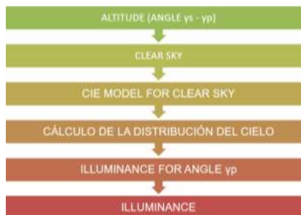
Figure 2 Schematic for calculating daylight availability ( \gamma_s solar altitude, \gamma_p altitude angle path in the sky), for clear or clear sky. CIE standard
