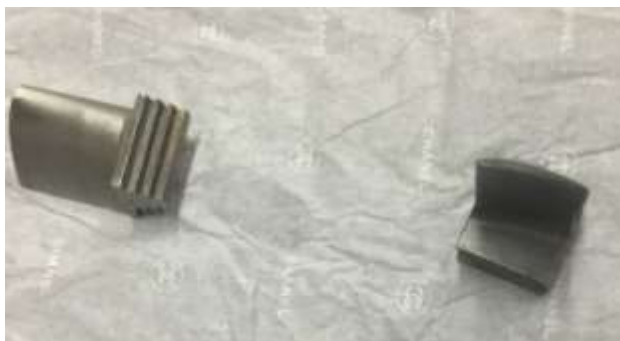
Figure 3 7th. Stage's blade, Rotor Axial Compressor
