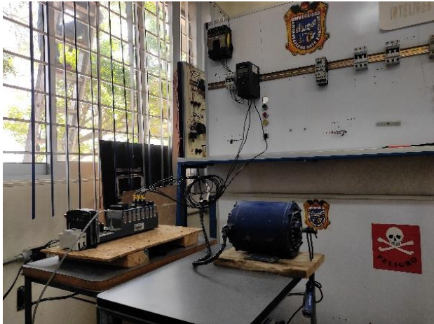
Figure 3 Three-phase motor speed control system
