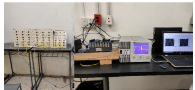
Figure 6 Data acquisition system connected to the RLC circuit.
