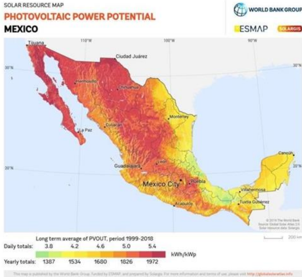
Figure 2 Map of Mexico with distribution of the municipalities with the highest radiation Source: https://solargis.com/es/maps-and-gis-data/download/mexico
