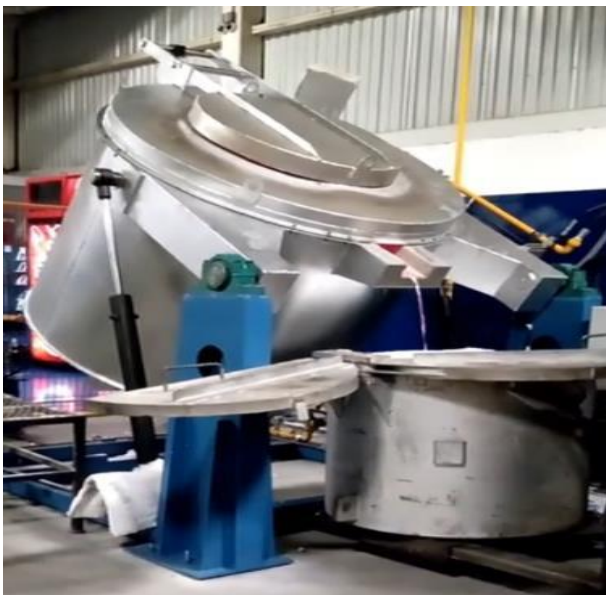
Figure 1 Melting furnace implementing: a) joint for tilting, b) joint for opening the lid
