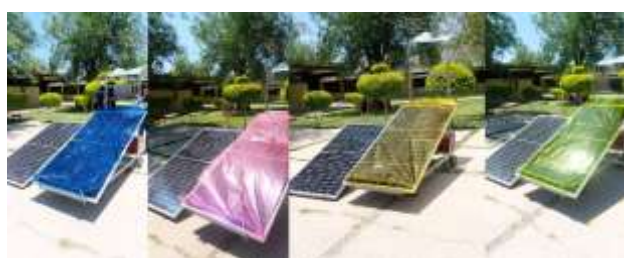
Figure 4 Blue, pink, yellow and lime green cellophanes installed in the VFM Own Elaboration
