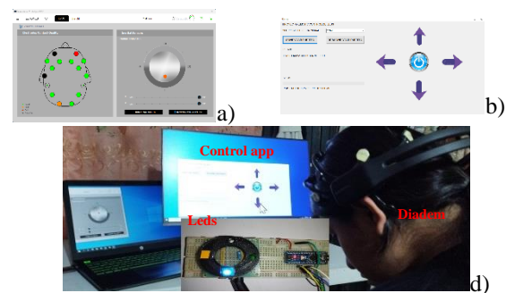
Figure 10 Inertial gyroscope method: (a) Xavier Control Panel software BCI interface, (b) motion control application and (c) head down
