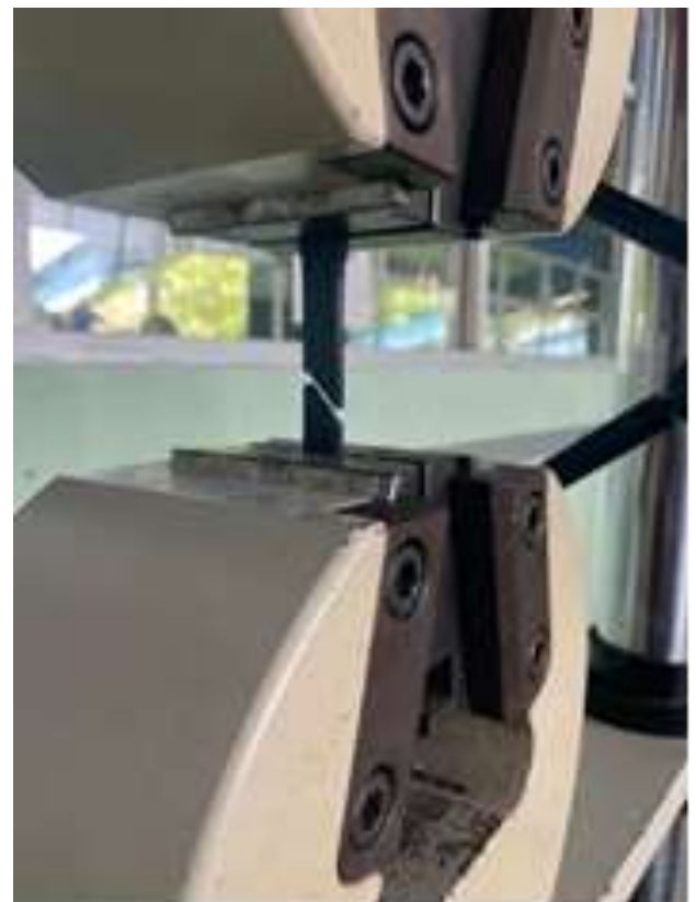
Figure 5 Tensile test on a type I specimen, made of ABS material
