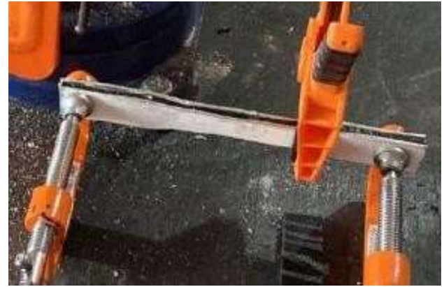
Figure 4 ABS test tube with reinforcement material (aluminum)
