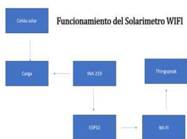
Figure 2 Operation of the Solarimeter Source: Own Elaboration (2023)
