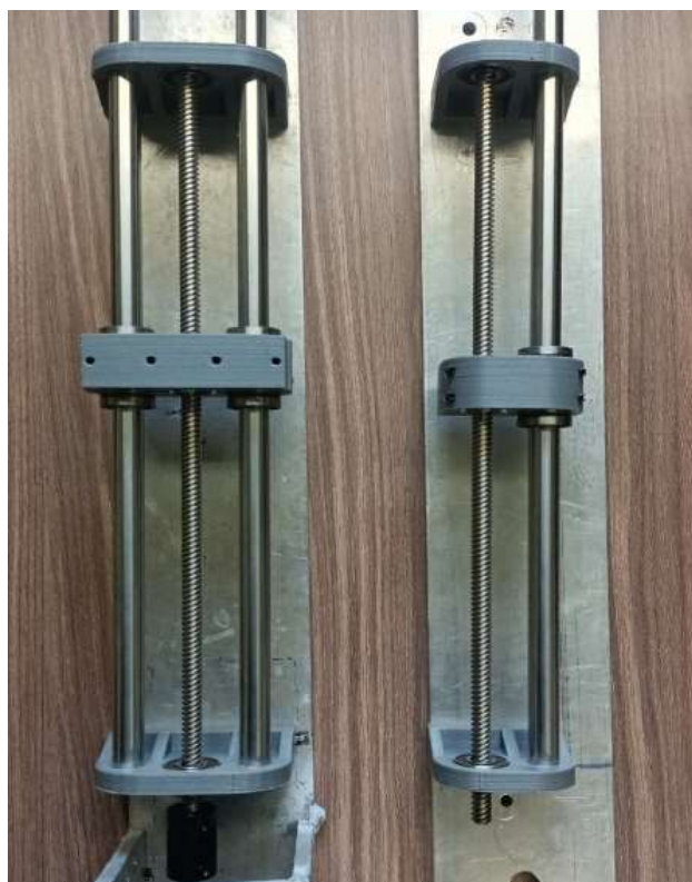
Figure 11 Final assembly of linear axis Source: Own Elaboration
