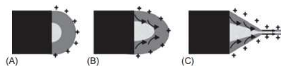
Figure 1 Schematic illustrating Taylor cone formation in the coaxial injector. A) Surface charges b) Shell formation in the droplet c) Taylor cone for shell formation
