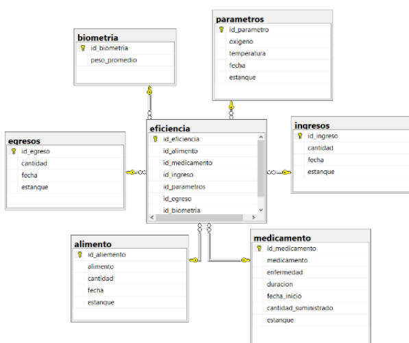
Figure 14 Data Warehouse of SIGETA in star-shaped schema Source: Own elaboration
