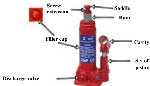
Figure 2 Parts of a bottle-type hydraulic jack
