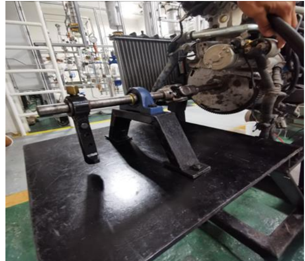
Figure 3 Dynamometer implemented in the test engine
