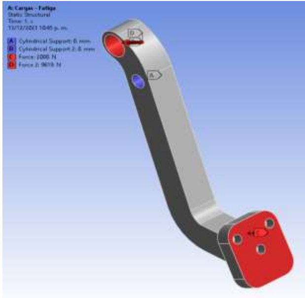
Figure 11 Global view of the pedal representing loads and supports exerted on the model for study
