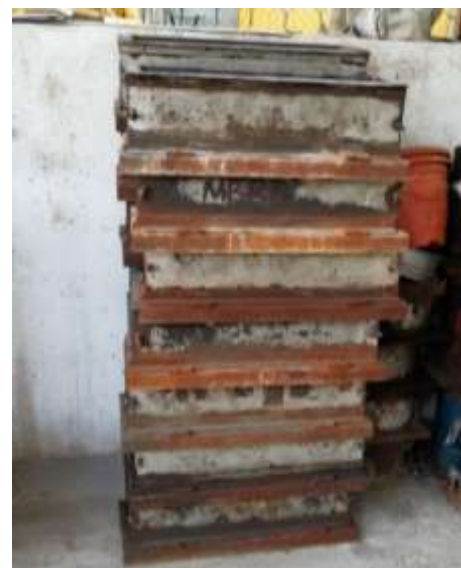
Figure 3 Concrete Beam Molds Source: Own elaboration (2021)
