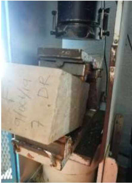
Figure 5 Testing of beams to obtain the MR. Source: Own Elaboration (2021)
