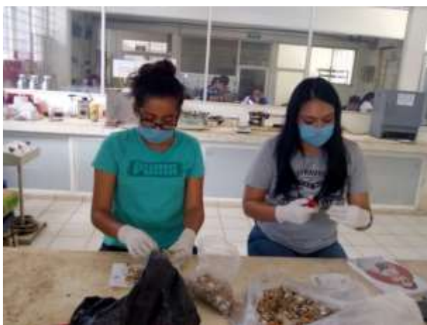
Figure 1 Obtaining and separating the fibers from cigarette butts
