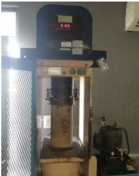
Figure 4 Cylinder test to obtain the f'_c Source: Own elaboration (2021)
