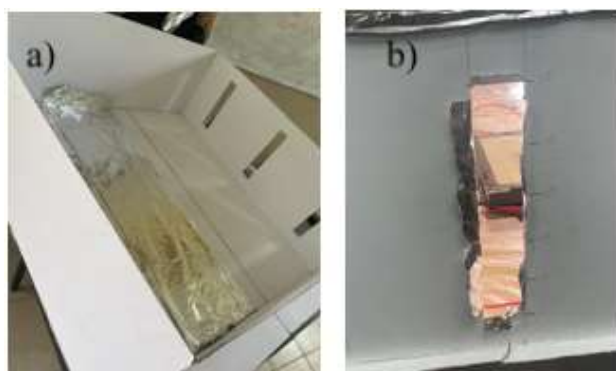
Figure 2 A) inside of the test box. B) opening for the introduction of the pyranometer
