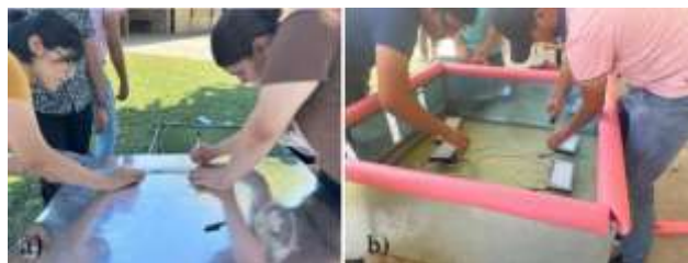
Figure 6 A) cutting of super polished sheet for solar simulator walls. B) fixing of lamps inside the box
