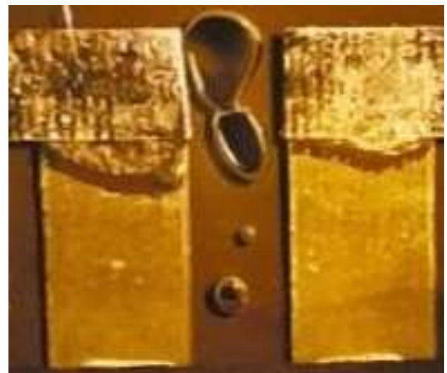
Figure 1 Plugs after Damp Heat Test
