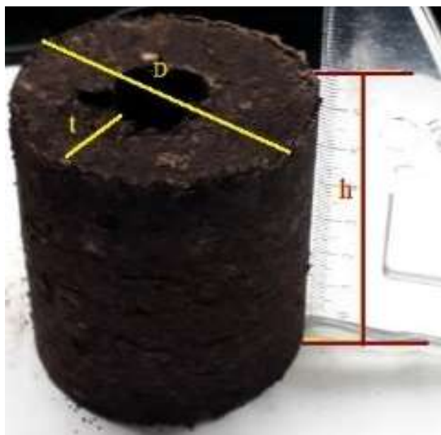
Figure 3 SCG-RNP briquettes dimensions Source: Own Elaboration
