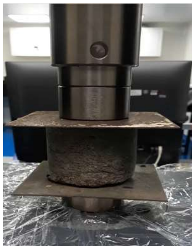
Figure 5 Compression strength test in universal testing machine Source: Own Elaboration
