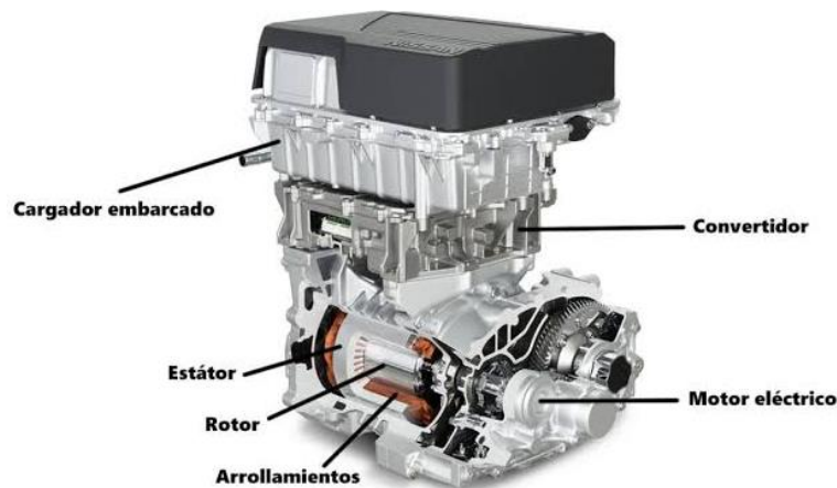
Figure 9.3 Components of an electric motor
