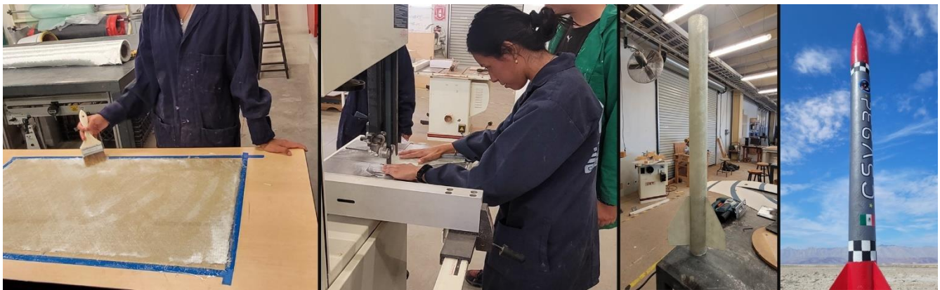
Figure 1.15 Model rocket manufacturing process. From left to right: Applying epoxy to fiberglass in order to manufacture fins of the rocket. Cutting the fiberglass to the desired form. Body of the rocket. Rocket fully painted
