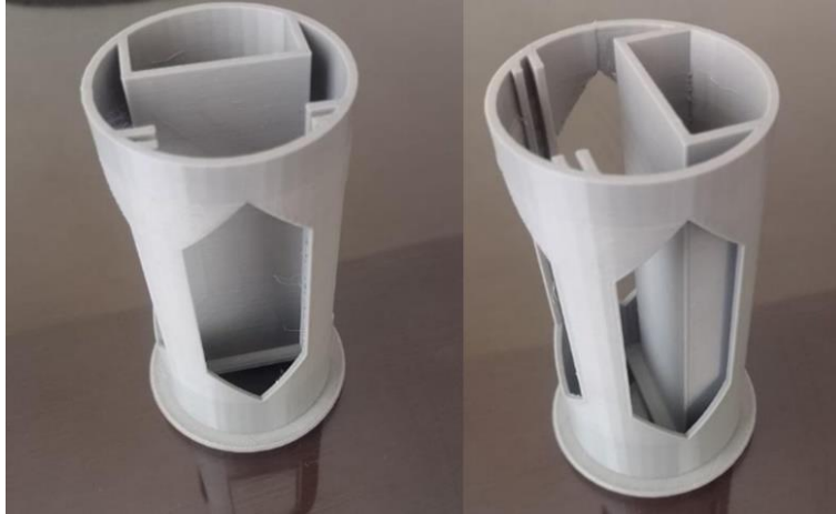
Figure 1.12 PLA container used for the structural subsystem
