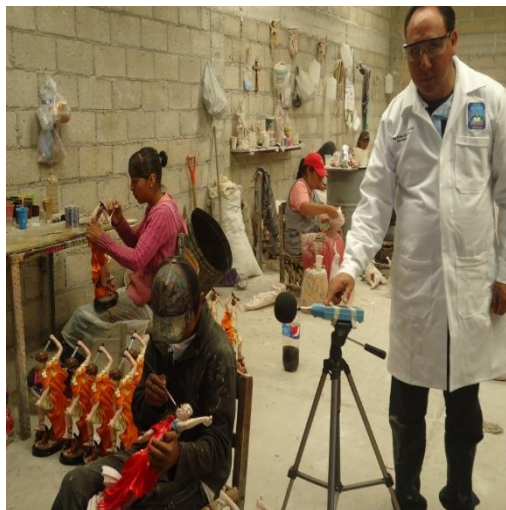
Figure 7.11 NSCEAT measurement with integrating sound level meter type 2, in the set-1 area
