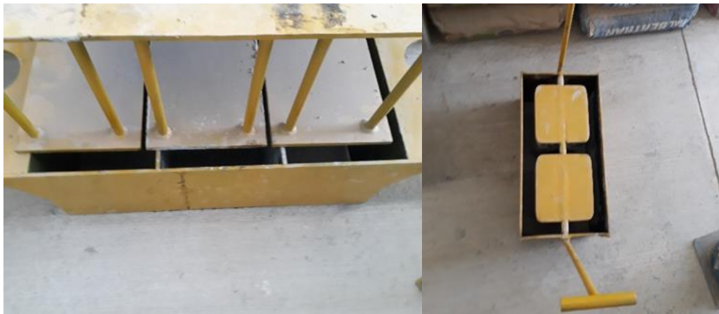
Figure 4.6 Commercial moulds to produce blocks 20 x 20 x 20 x 40 cm
