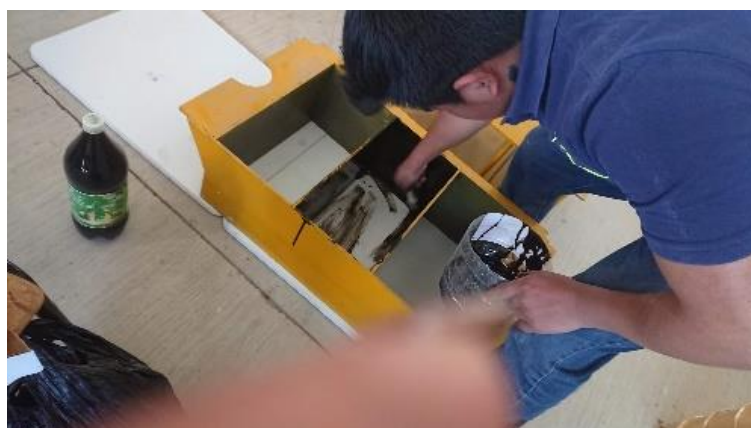
Figure 4.7 Application of burnt oil to the metal mould
