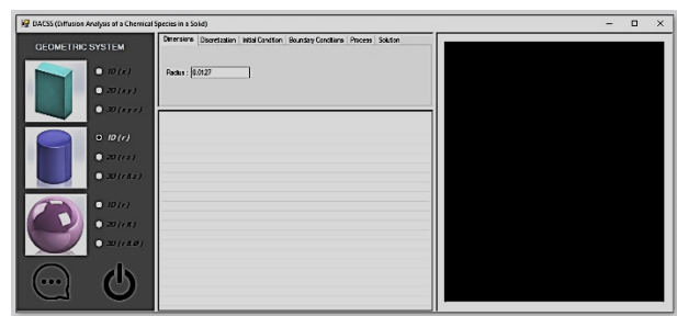
Figure 4 Graphical user interface developed for calculating carbon concentration histories and profiles in the carburization process Source: Image by screenshot of the development in MS Visual Studio Express 2010.
