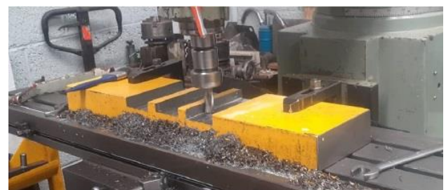
Figure 10 Moving part grooving process Source: Own design.
