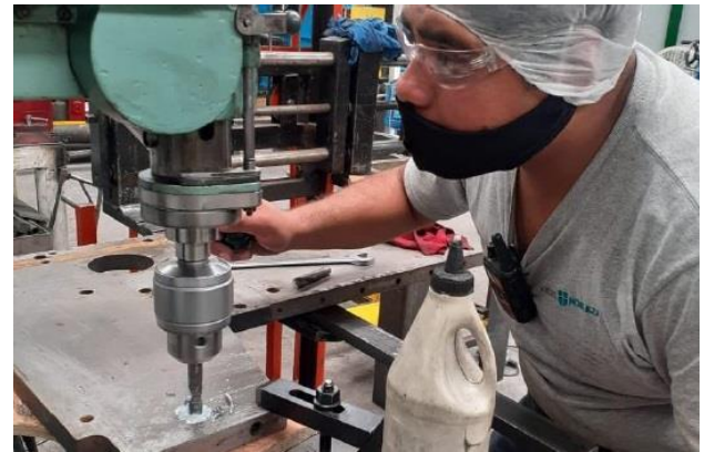
Figure 9. Plate drilling Source: Own design
