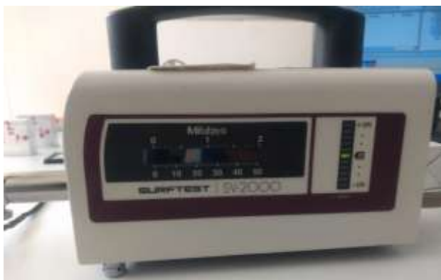
Figure 6 Mitutoyo SURFTEST SV-2000 roughness tester
