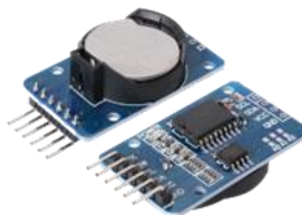
Figure 6 RTC module DS3231
