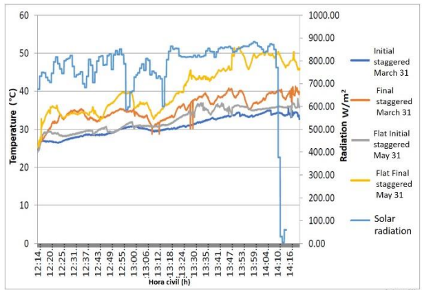
Figure 4 Temperature increase in CaCl 2 regeneration equipment
