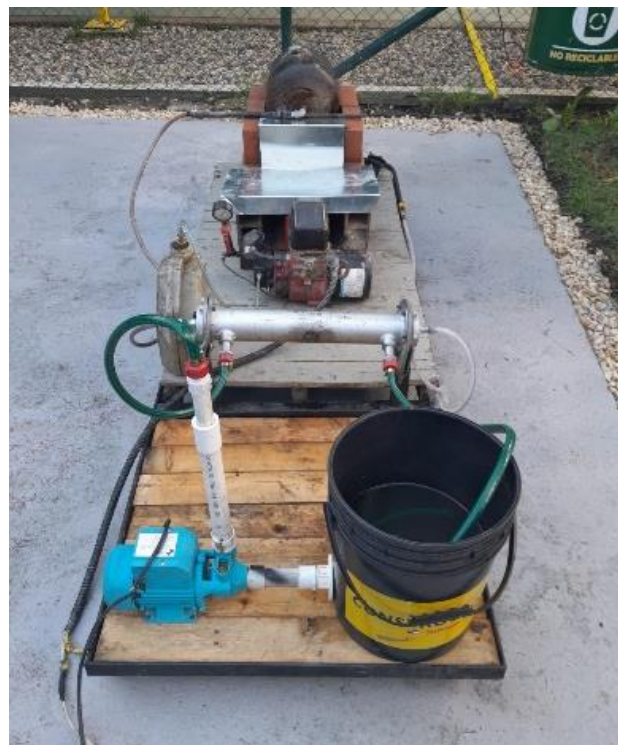
Figure 4. Rubber pyrolysis equipment Source: Own Elaboration
