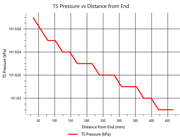
Figure 10 Pipe side pressure drop Source: Own Elaboration
