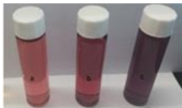
Figure 6 Color of the AuNPs solutions prepared with the aqueous extract of Stevia rebaudiana at different reaction times, a) 30 min, b) 2 h, c) 4 h. Source: author's own
