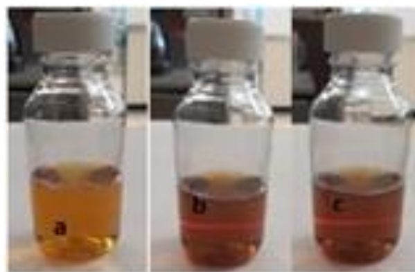
Figure 2 Color of the solutions of the AgNPs at different times from the beginning of their formation reaction: a) 30 min, b) 60 min, c) 90 minutes
