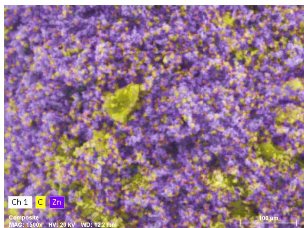
Figure 5 SEM mapping for C (yellow) and Zn (purple) Source: Own elaboration
