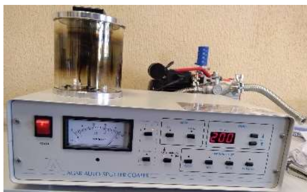
Figure 3 Surface coating equipment by sputtering, AGAR AUTO SPUTTER COATER, Model 108a
