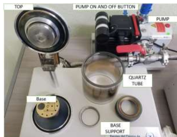
Figure 4 View from above of the sputtering system used for the deposition of the nanoparticles
