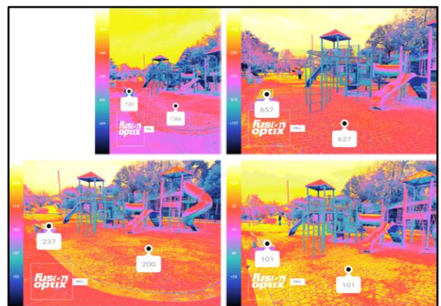
Figure 7 Luminance maps 14:00, 15:00, 16:00 and 17:00h at points 5 and 6 Source: Miriam Mery-Ruiz. 2023. Photographs taken with Fusion Optix app
