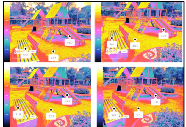
Figure 11 Luminance maps 14:00, 15:00, 16:00 and 17:00h at point 12 Source: Miriam Mery-Ruiz. 2023. Photographs taken with Fusion Optix app.
