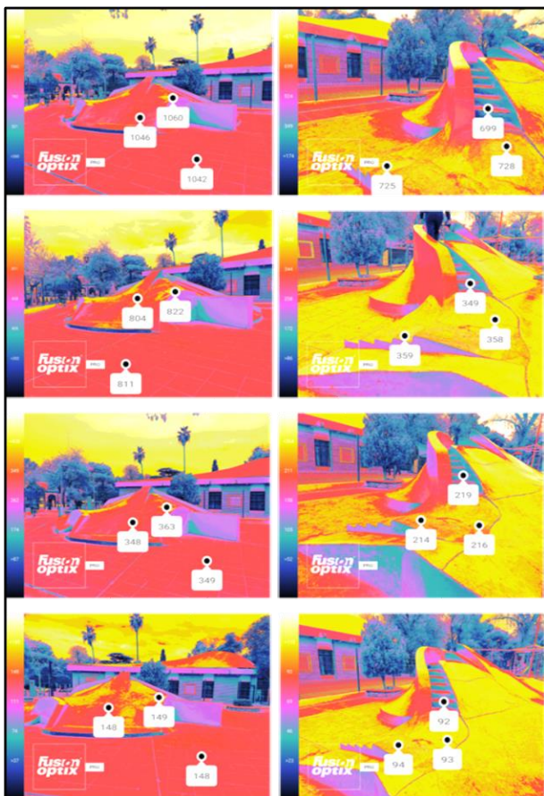
Figure 9 Luminance maps 14:00, 15:00, 16:00 and 17:00h at points 8, 9 and 10
