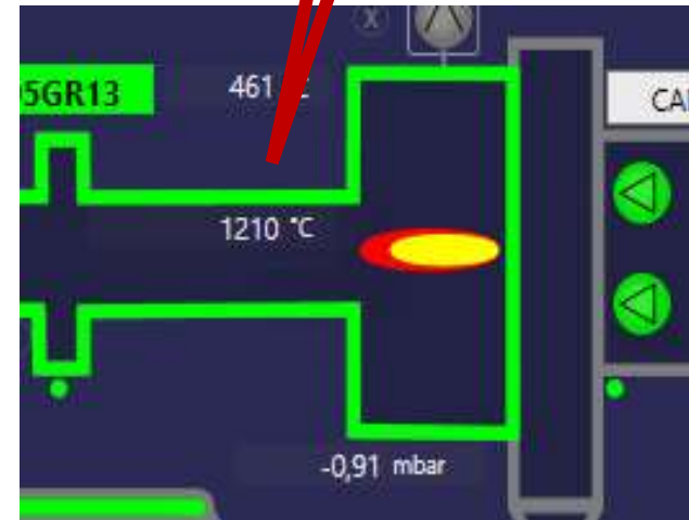
Figure 6 Operating screen mimic, furnace temperature analyzer. Taken from own image
