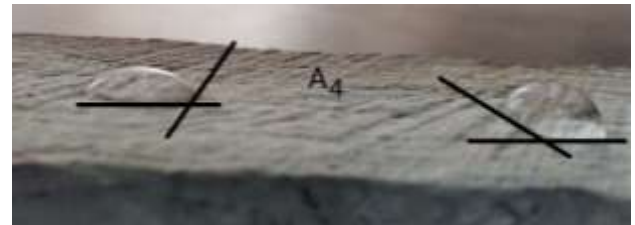
Figure 4 Contact angle of A4 with H 2 O and HCl. Source: Own Elaboration
