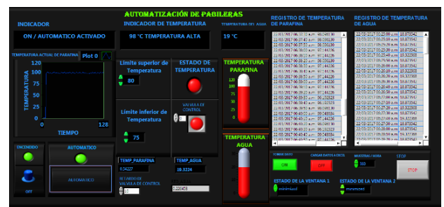
Figura 6 Panel de control
