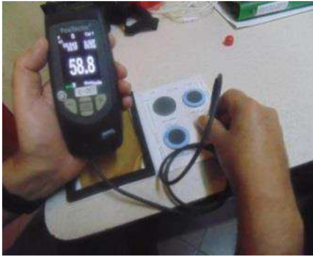
Figure 2 Individual readings on Coated Plate (28945) located in the Coating Thickness Standards Source: Own Elaboration
