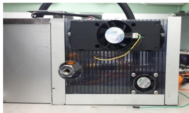
Figure 11 Regulation and cooling system for water in the thermal cycler
