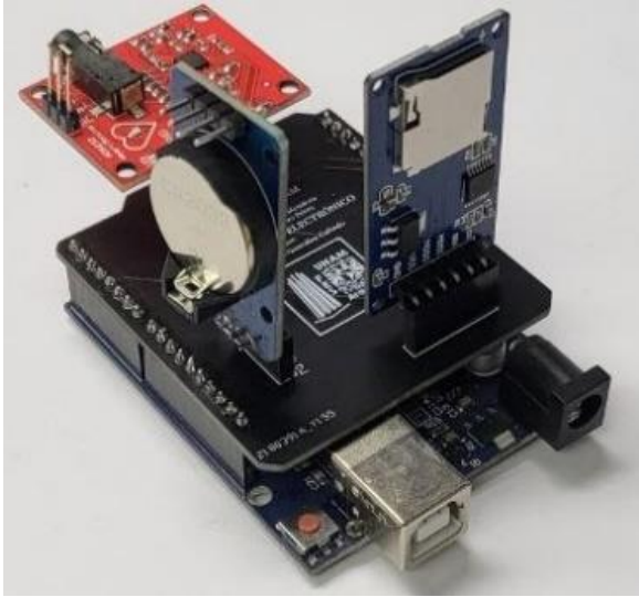
Figure 14 Printed circuit board with the assembled modules on the Arduino UNO development board
