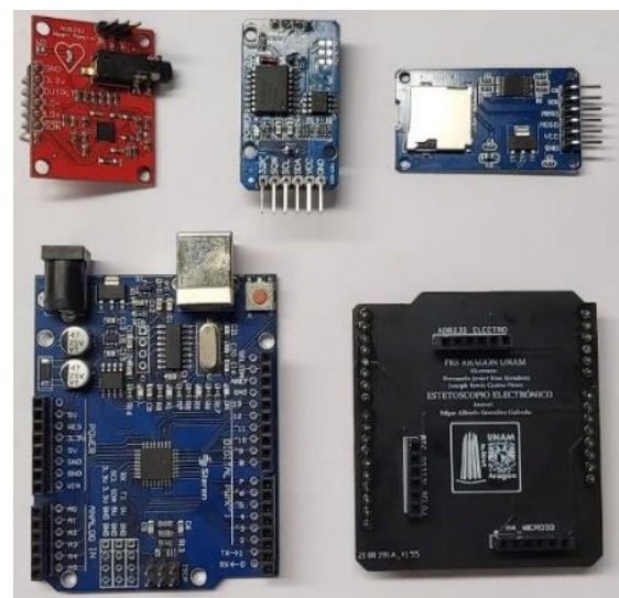
Figure 13 AD8232, RTC-DS3132 and microSD card reader modules, together with development board and PCB
