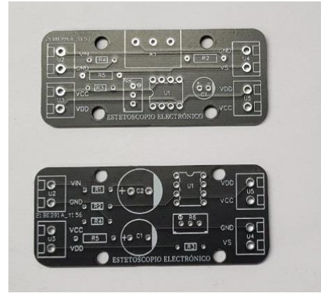
Figure 7 Active 2nd Order Low Pass Filter and Preamplifier PCB
