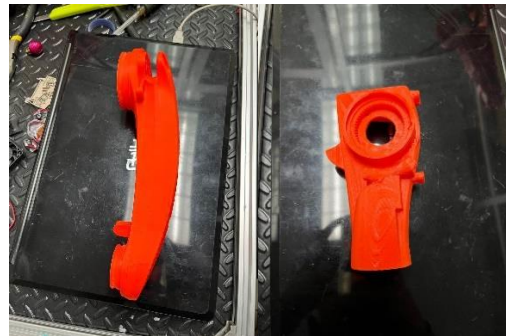
Figure 11 3D printed parts (oscillator arm and neutral arm)
