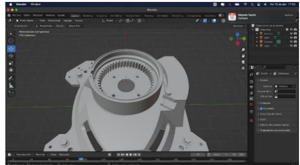
Figure 1 3D model of the robot (planetary gearing system)
